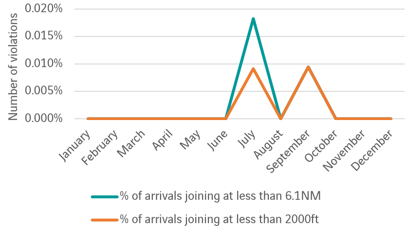
Figure 24: Day time joining point violations
